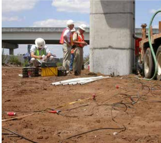
**Figure 7:** SR data being collected along pier foundations for elevated roadway.
