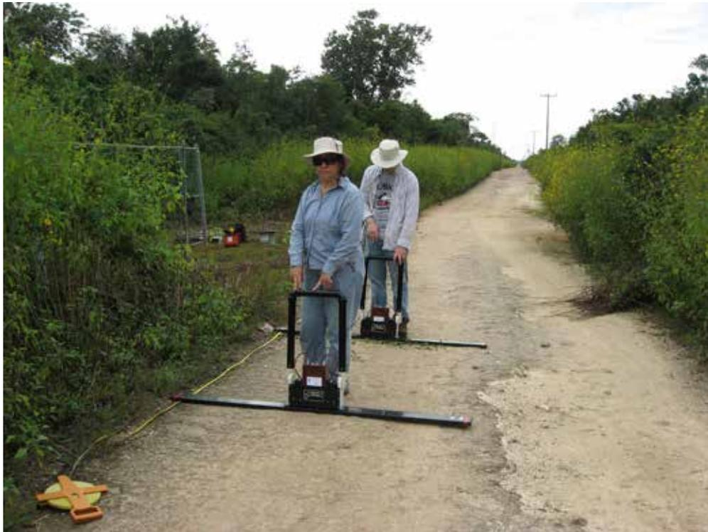
**Figure 4:** GPR surveys along a wellfield service road near Well 49A (Area 1). Surveys off the roads were not feasible due to heavy jungle. Sources of interference such as chain-link fences and powerlines (shown here in the distance) were noted in the field and identified on adjacent GPR sections, so as not to misidentify them as legitimate reflectors.
