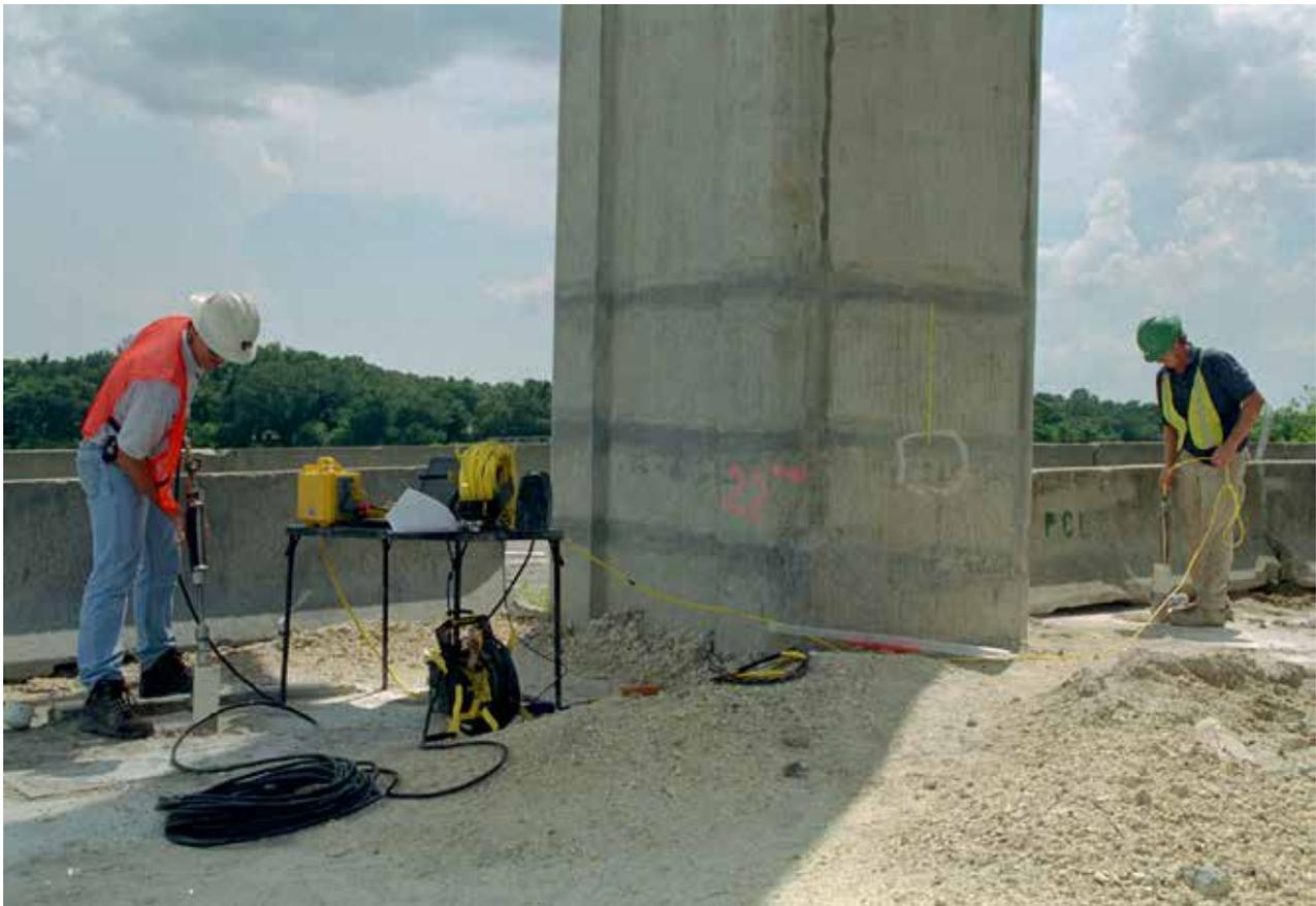
**Figure 9:** Crosshole seismic data being collected up to 40 ft below bottom of shafts.
