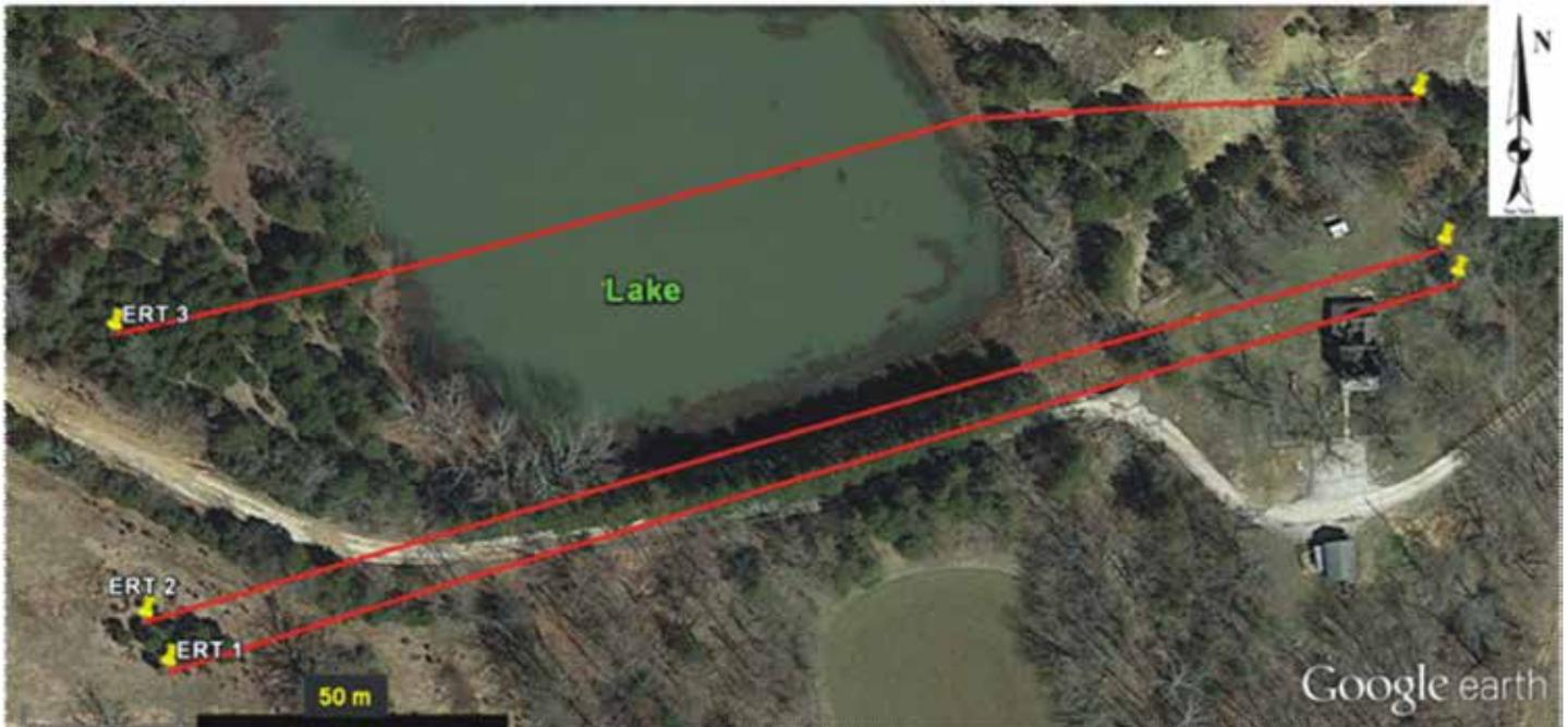
**Figure 1:** Google earth image of the earthfill dam showing upstream lake and the locations of ERT traverses 1-3 (Figure 3).
